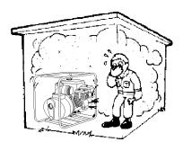
flow is restricted it will cause serious damage to the pump or engine and may cause injury to people and property. Remember the pump's engine gives off **DEADLY** gases.
